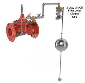
The CLA-VAL SERIES 100 On/Off Float Level Control Valve is a non-modulating valve which accurately controls the liquid level in a tank. This valve opens fully when the liquid level reaches a preset low level and closes drip tight when the liquid level reaches a high level.
