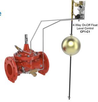
The CLA-VAL SERIES 100 On/Off Float Level Control Valve is a non-modulating valve which accurately controls the liquid level in a tank. This valve opens fully when the liquid level reaches a preset low level and closes drip tight when the liquid level reaches a high level.
