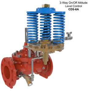
The CLA-VAL SERIES 210 On/Off Altitude Level Control Valve controls the high water level in a reservoir or closed tank without the need for floats or other devices. It is a non-throttling valve that remains fully open until the shut-off point is reached.
