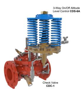
The CLA-VAL SERIES 210 On/Off Altitude Level Control Valve controls the high water level in a reservoir or closed tank without the need for floats or other devices. It is a non-throttling valve that remains fully open until the shut-off point is reached.
