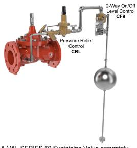
The CLA-VAL SERIES 50 Sustaining Valve accurately maintains a minimum preset (Pressure Relief Control) inlet pressure regardless of changing flow rate. The CLA-VAL SERIES 50 Relief Valve opens fast to dissipate excess system pressure.
