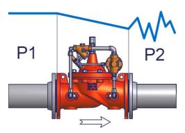
The CLA-VAL SERIES 50 Relief Valve opens fast to dissipate excess system pressure.
