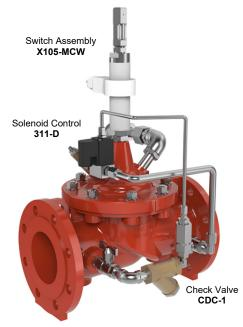
The CLA-VAL SERIES 60 Pump Control Valve is a pilot-operated valve designed for installation on the discharge of pumps to prevent pipeline surges caused by starting and stopping of pumps.
