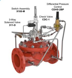
The CLA-VAL SERIES 60 Pump Control Valve is a pilot-operated valve designed for installation on the discharge of pumps to prevent pipeline surges caused by starting and stopping of pumps.
