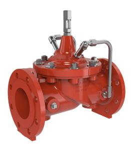
The CLA-VAL SERIES 81 is a hydraulically operated Check Valve. The valve opens when inlet pressure exceeds outlet pressure. In case of reversal pressure, the higher outlet pressure closes the valve to prevent backflow through the valve.
