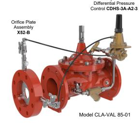
The CLA-VAL SERIES 85 is an excess flow or excess pressure shut-off valve. When flow or pressure reaches a preset value, the valve closes.
