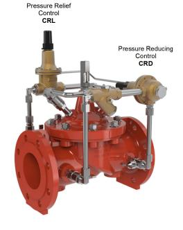
The CLA-VAL SERIES 90 reduces a higher inlet pressure to a constant downstream pressure (Pressure Reducing Control) regardless of changing flow rate and/or varying inlet pressure.
