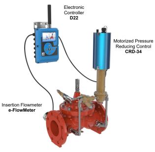
The CLA-VAL SERIES D22 programmable Control Valves automatically adjust valve regulation according to customized pre-defined rules.
