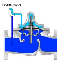
Full Open Operation: When pressure in the cover chamber is relieved to a lower pressure or to atmosphere, the pressure inlet opens the valve.
