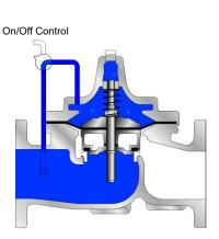
Tight Closing Operation: When pressure from the inlet pressure is applied to the cover chamber, the valve closes driptight.
